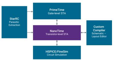
Transistor-level Static Timing Analysis
